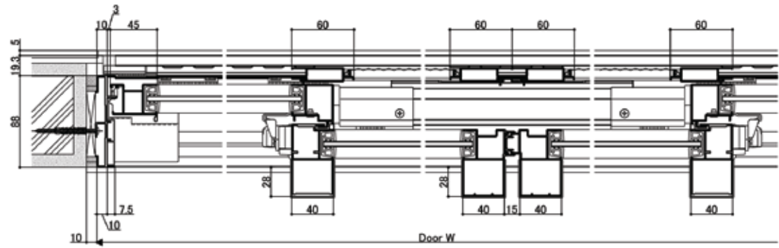
< Horizontal section: With optional flat-sill attachment Outside >
