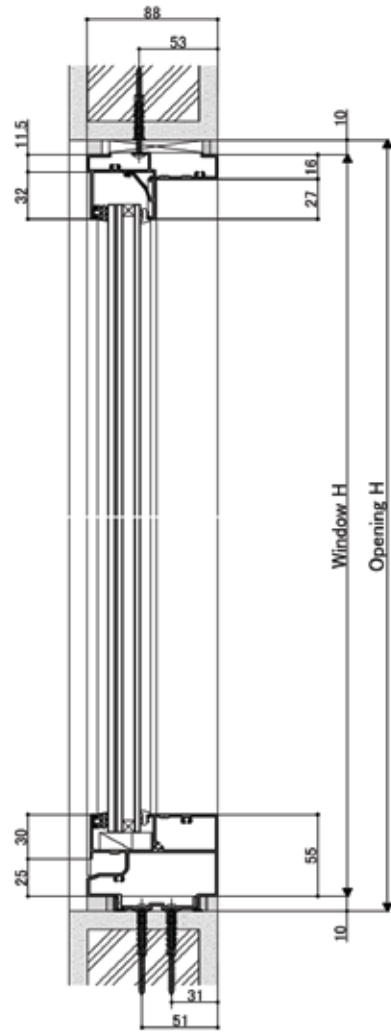
< Vertical section: Single fixed window (IG unit) >
