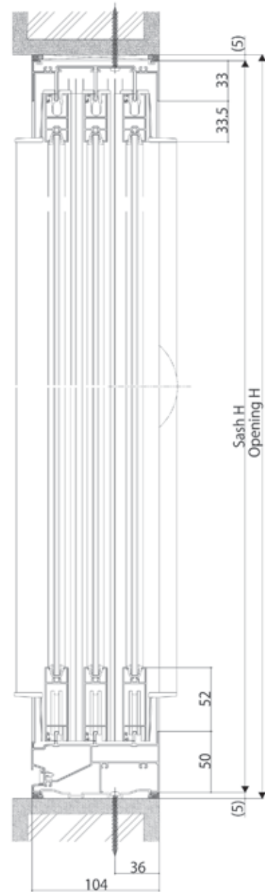
< Vertical section: 3 panels sliding window >
